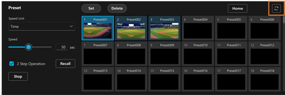
Click the preset update button (area in the above figure surrounded by a bounding box) to load the latest preset from the camera and update the screen display.
