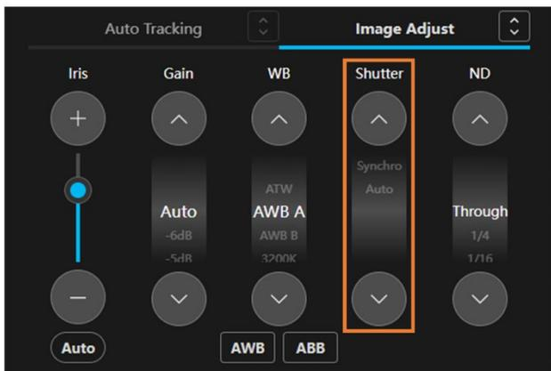
The Shutter mode for the camera can be configured with the Shutter part (area in the above figure surrounded by a bounding box) in the camera controller Image Adjust operator.
