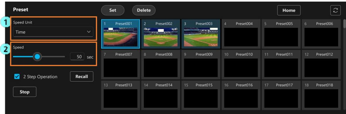
1. With [Speed Unit], you can select the unit used for preset movement speed.
