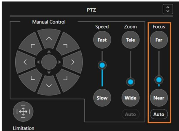
The Focus for the camera can be adjusted with the Focus part (area in the above figure surrounded by a bounding box) in the camera controller PTZ operator.
