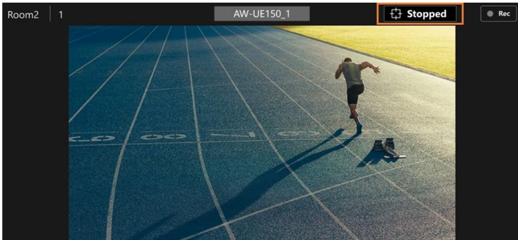
The tracking status during Auto Tracking is displayed at the top right of the camera view area.
