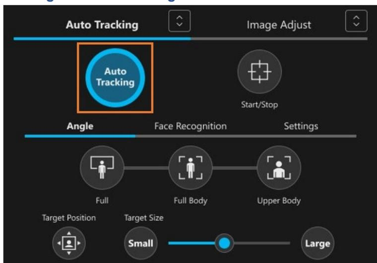
You can turn the Auto Tracking Function ON/OFF with the [Auto Tracking] button (enclosed within a frame in the figure above) in the Auto Tracking control panel of the camera controller.
