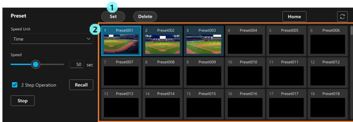
1. Click the [Set] button in the preset operator to turn the button ON.
