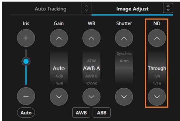
The ND Filter for the camera can be configured with the ND part (area in the above figure surrounded by a bounding box) in the camera controller Image Adjust operator.
