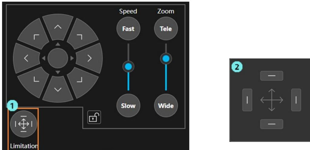
Click the [Limitation] button (Fig. 1 above) in the PTZ control panel to display the Pan/Tilt range setting panel (Fig. 2 above).
