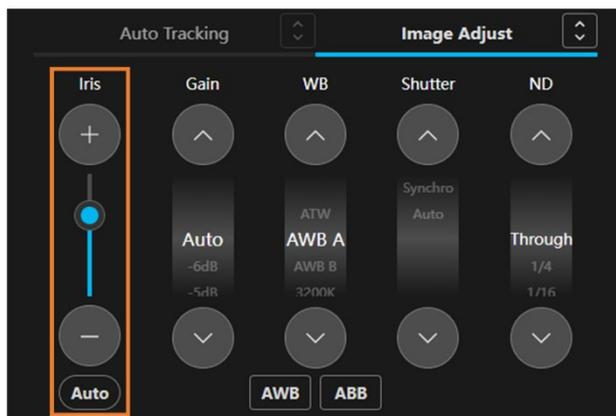
The Iris for the camera can be adjusted with the Iris part (area in the above figure surrounded by a bounding box) in the camera controller Image Adjust operator.
