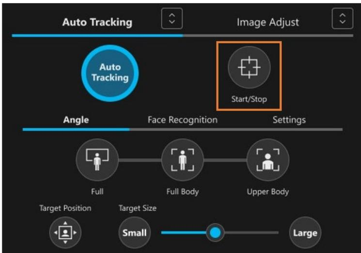
You can start or stop the camera movement using Auto Tracking with the [Start/Stop] button (enclosed within a frame in the figure above) in the Auto Tracking control panel of the camera controller.
