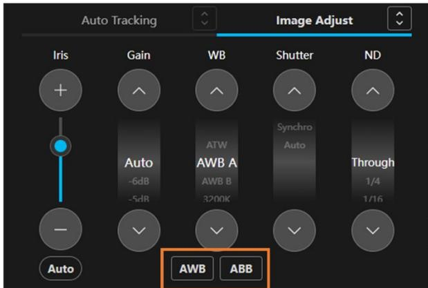
Click the [AWB] button in the camera controller Image Adjust operator to execute AWB on the camera. Click the [ABB] button to execute ABB on the camera.
