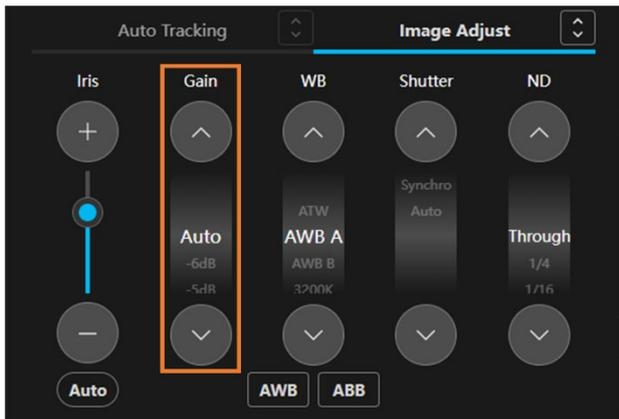
The Gain for the camera can be configured with the Gain part (area in the above figure surrounded by a bounding box) in the camera controller Image Adjust operation part.
