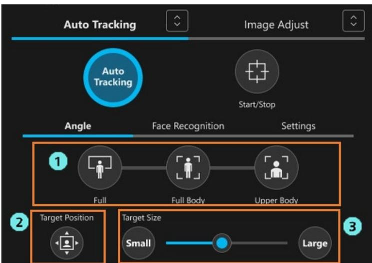
You can set the camera angle during Auto Tracking with the [Full] button/[Full Body] button/[Upper Body] button (Fig. 1 above) under the [Angle] tab in the Auto Tracking control panel of the camera controller.
