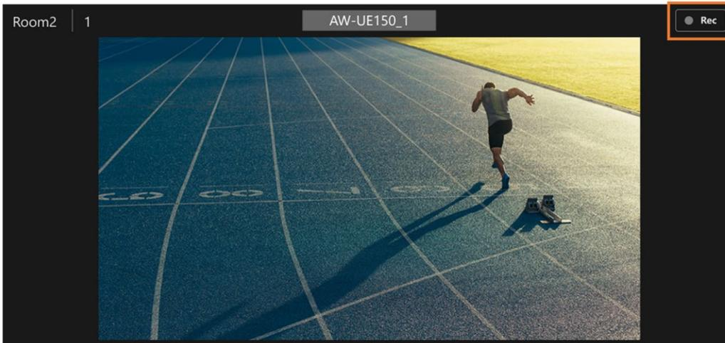
If the camera supports the video recording function, you can click the [Rec] button (area in the above figure surrounded by a bounding box) in the camera video area to start and stop video recording on the camera.
