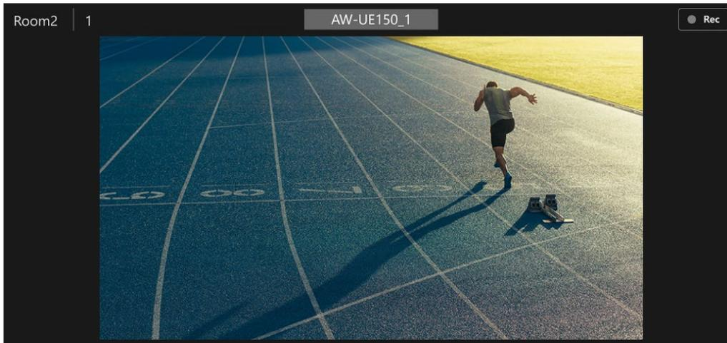
Click anywhere in the camera's video to pan and tilt the camera with that position as the center of focus.
