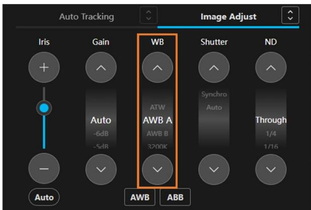
The White Balance mode for the camera can be configured with the WB part (area in the above figure surrounded by a bounding box) in the camera controller Image Adjust operator.
